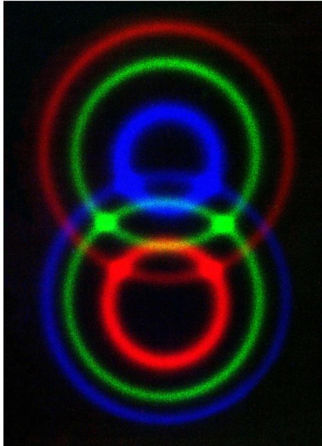
**Figure 5.** A photograph of the down-conversion photons, taken with different interference filters. Photo: Michael Reck and Paul Kwiat.
