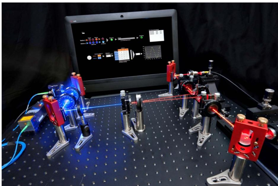
**Figure 18.** The source of entangled photon pairs used in the test of Bell's inequality at dOCUMENTA (13). Photo: Lois Lammerhuber.
