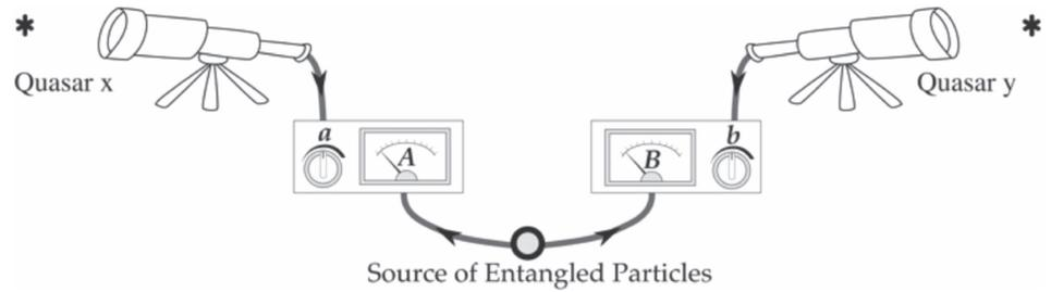
**Figure 23.** Proposal for a Cosmic Bell experiment. Two telescopes observe distant objects, for example, two quasars. The random fluctuations in the light obtained from the quasars are used to set the polarizers in a Bell inequality experiment. These quasars are probably the most independent sources of randomness one can have in the Universe. Reprinted with permission from [82]. Copyright (2014) by the American Physical Society.
