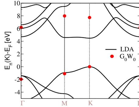
**Figure 3.** The band structure of hBN-ML obtained by the LDA. The red dots represent the q2D- $G_0W_0$  correction of highest occupied (valence) and the lowest unoccupied (conduction) bands in  $\Gamma$ , K and M points of Brillouin zone.
