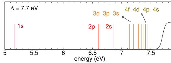
**Figure 5.** The excitonic spectrum of hBN-ML containing first ten levels (solid lines) from the table 1. The dashed maroon line represents the exciton ground state energy  $\Omega_{1s}(\lambda_{\text{DFT}}) = -2.53$  eV calculated using the  $\lambda_{\text{DFT}}$  static screening length. The threshold energy for the single particle excitations is represented by a black line.
