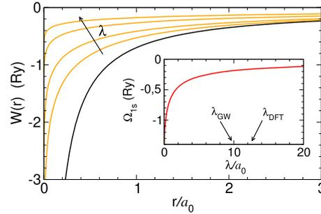
**Figure 4.** The bare Coulomb potential (black) and the screened Coulomb potential (2.29) (orange) plotted for different parameters  $\lambda = 1, 2, 5, 10a_0$ . The insert shows dependence of the ground state exciton binding energy  $\Omega_{1s}$  on  $\lambda$  for  $\mu = 0.35m_e$ .
