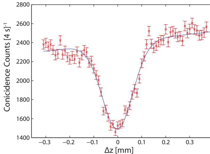
**Figure 5.** Example of observed two-photon interference between output waveguides 2 and 6 as a function of relative path difference between photon pairs input into neighbouring waveguides 1 and 2. The visibility of the dip is  $\mathcal{V}_{2,6} = 38 \pm 2\%$ , calculated from a Gaussian fit (blue line).
