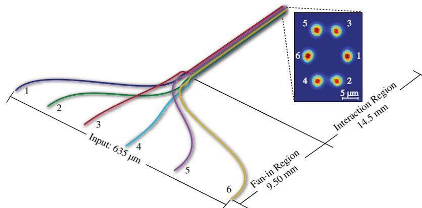
**Figure 1.** Schematic representation of the integrated waveguide circuit (drawing not-to-scale) and associated output. At the input the waveguides are equally spaced by  $127 \mu\text{m}$ . They then converge via a two-stage fan-in to their eventual elliptical configuration. The inset is a CCD image of the output: the waveguides are arranged with equal angular spacing around an ellipse with semi-major and semi-minor radii of  $10.2$  and  $7.0 \mu\text{m}$ , respectively.
