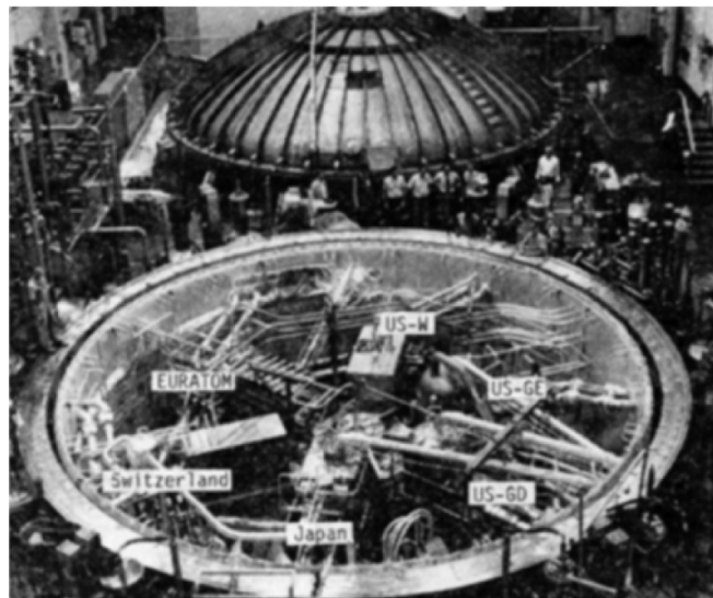
Figure 4. Six LCT coils in a vacuum tank (October 1985).
