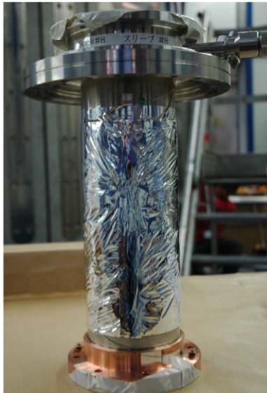
Figure 12. A picture of the cold-heads with sock enveloped in three layers of MLI.
