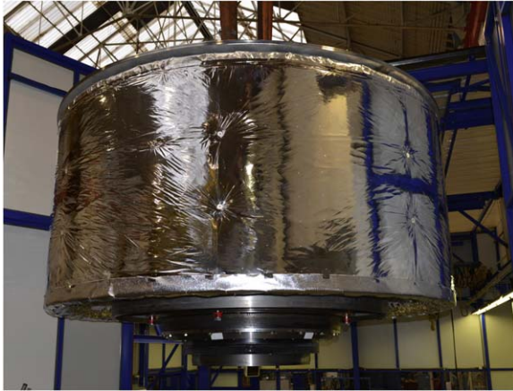
Figure 13. Photograph of the EcoSwing rotor enveloped in three MLI blankets.
