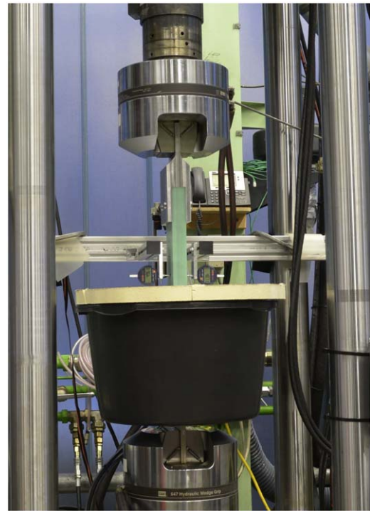
Figure 11. Photograph of one subscale CWS that was mechanically load tested with one side at room temperature and the other in liquid nitrogen.
