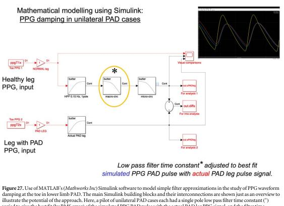
varied to give the best fit (by RMS error) of the simulated PPG PAD pulse with the actual PAD leg PPG signal, and the filter time constants compared with a reference standard for PAD such as the ABPI. Such pilot experiments can form a starting point for better understanding the damping and timing of PPG with disease. More detailed studies could include the analysis of ambulatory/wearable PPG signals for PAD diagnostics.
