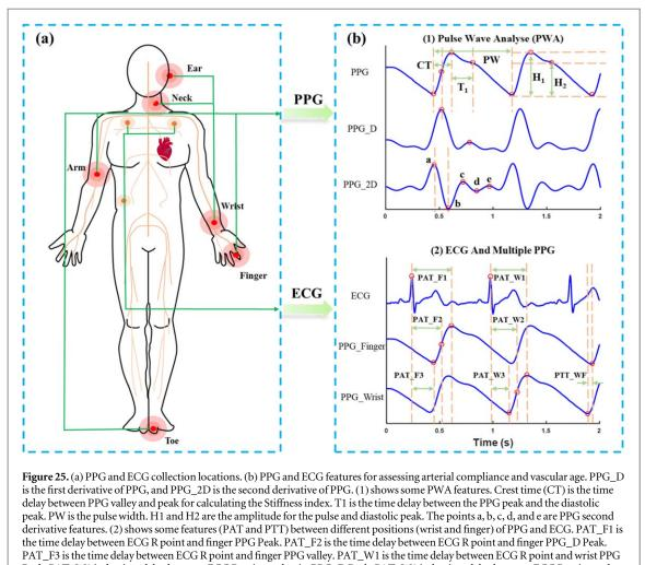
Peak. PAT\_W2 is the time delay between ECG R point and wrist PPG\_D Peak. PAT\_W3 is the time delay between ECG R point and wrist PPG valley. PTT\_WF is the time delay between finger PPG valley and wrist PPG valley.
