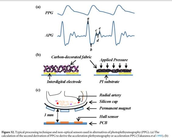
**Figure 32.** Typical processing technique and non-optical sensors used in alternatives of photoplethysmography (PPG). (a) The calculation of the second derivation of PPG to derive the acceleration plethysmography or acceleration PPG (Takazawa *et al* 1998). (b) A piezoresistive sensor for obtaining the impedance PPG (modified from Luo *et al* (2016)). (c) A series of Hall sensors for capturing the magnetic induction plethysmography (modified from Kim *et al* (2018)).
