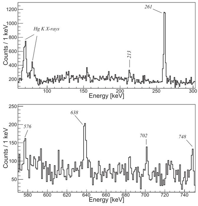
**Figure 5.** Part of the  $\gamma$ -ray spectrum in  $A = 182$ , background-subtracted, with a gate on the  $K$  electron of the  $0_2^- \rightarrow 0_1^-$   $E0$  transition in  $^{182}\text{Hg}$ . The top and bottom panels show the spectrum in a different energy range.
