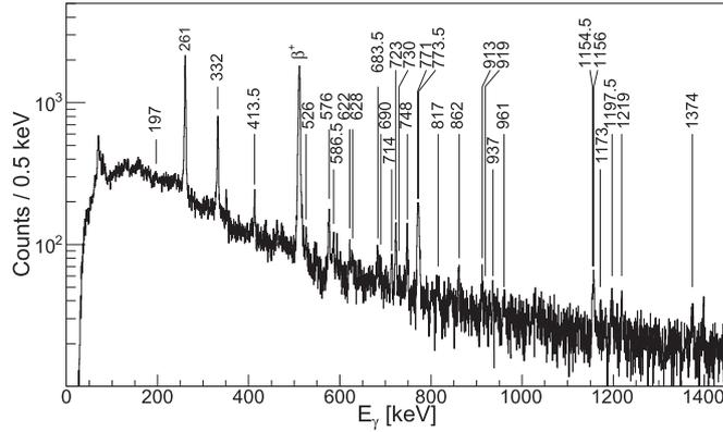
**Figure 3.** The  $\gamma$ -ray spectrum coincident with the 351 keV  $2_1^+ \rightarrow 0_1^+$  transition in  $^{182}\text{Hg}$ . The labels in the spectrum give the energy of the transitions in keV.
