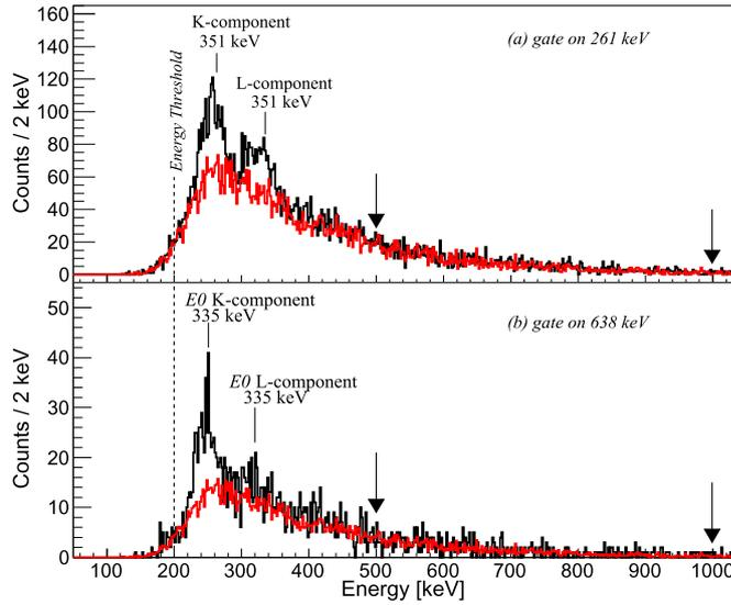
**Figure 6.** Si spectrum at  $A = 182$  gated on (a) the 261 keV transition and (b) the 638 keV transition. The red curve shows the  $\Delta E$  spectrum due to the  $\beta$  particles. The arrows indicate the energy range used to normalize the  $\beta$ -ray spectrum to the  $\gamma$ -gated Si spectrum.
