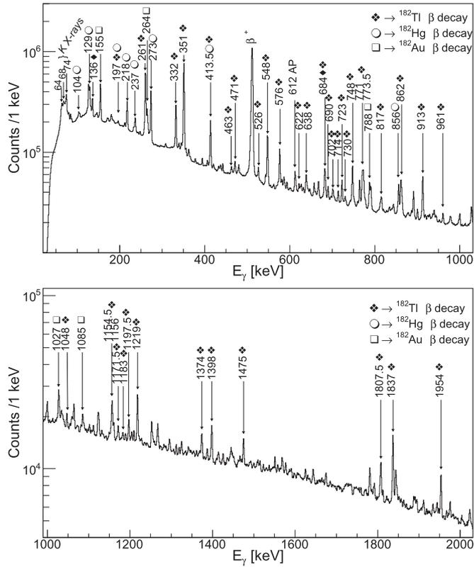
**Figure 2.**  $\gamma$ -ray singles spectrum obtained at  $A = 182$  by the Ge1 detector. Transitions assigned to the decay of  $^{182}\text{Tl}$  are indicated, together with some identified transitions belonging to daughter nuclei. The other lines are due to room background or residual radioactivity due to previous implantations. The numbers next to the peaks give the energies in keV.
