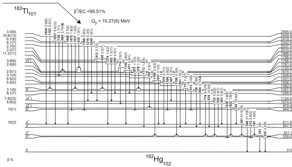
**Figure 4.** Level scheme of  $^{182}\text{Hg}$  deduced from the present work (energies in keV). The  $\gamma$ -ray intensities and the intensity of the 335 keV  $E0$  transition are normalized to the 351 keV ( $2_1^+ \rightarrow 0_1^+$ ) transition. The given  $\beta$ -feeding intensities are upper limits. Spin assignments are from NNDC [20] except for the ( $2^+$ ) assignment of the 973 keV level (see discussion in the next section). The  $Q_{EC}$  value comes from [21].
