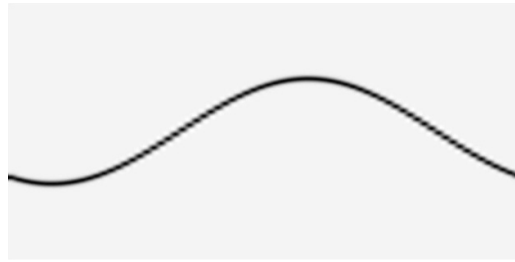
Figure 4. The sinogram of a very small Gaussian, sampled at 5^\circ in \varphi , then interpolated. In the steep parts of the curve, the interpolation is not optimal but it is good along the horizontal ones.
