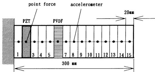
**Figure 4.** The division of the cantilever beam.
