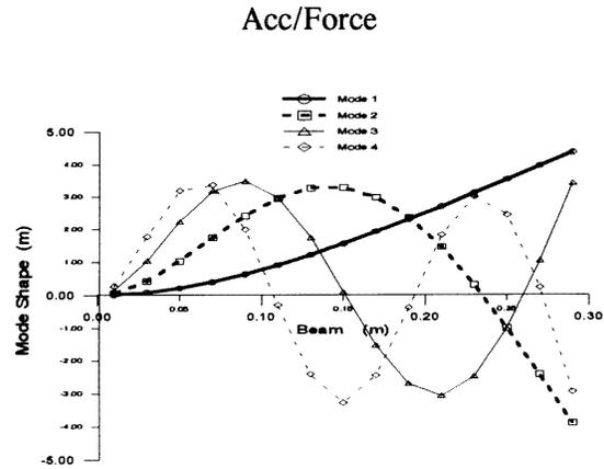
**Figure 9.** The prediction of the mode shapes from SMA for Acc–Force.
