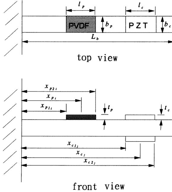
Figure 2. The piezoceramic transducers on the cantilever beam.
