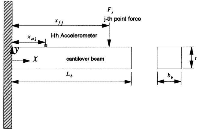
Figure 1. The conventional transducers on the cantilever beam.
