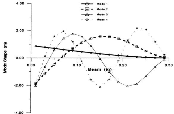
**Figure 6.** The theoretical mode shapes of the piezoceramic transducers.
