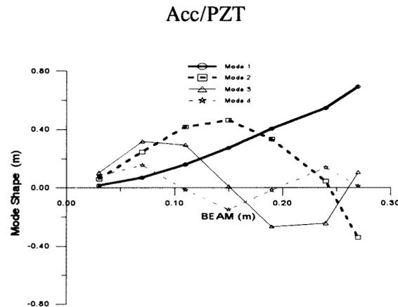
**Figure 10.** The prediction of the mode shapes from SMA for Acc–PZT.
