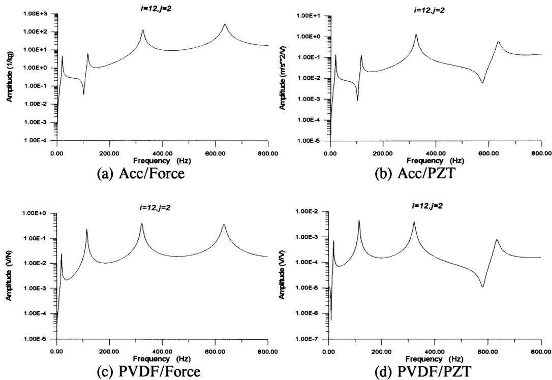
Figure 8. Theoretical transfer frequency response functions for  $i = 12$  and  $j = 2$ .
