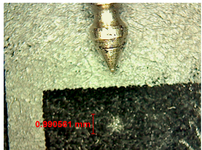
Figure 11. Damage induced by a multimeter probe on GO paper during an attempt to measure its resistive value.
