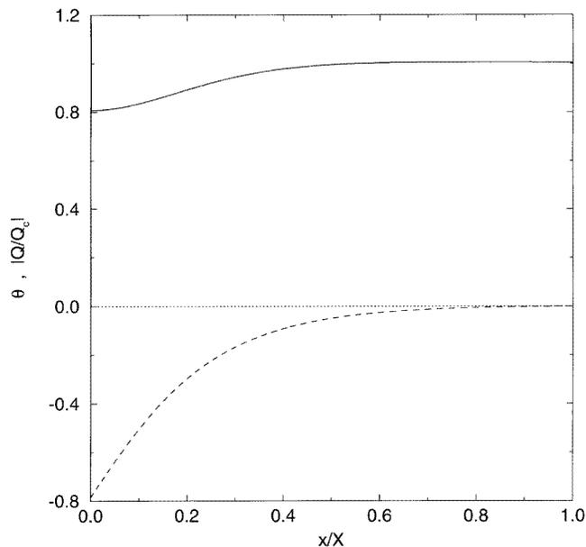
**Figure 1.** The reduced amplitude  $|Q/Q_c|$  (solid line) and phase  $\theta$  (dashed line) of the IC order parameter as functions of  $x/X$  for  $r = 0.44$  (the value for  $\text{Cs}_2\text{ZnI}_4$ ) at a temperature just above the IC–C transition. The point  $x = 0$  is at the centre of a discommensuration and the point  $x = X$  is mid-way between two discommensurations.
