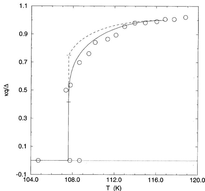
**Figure 2.** The reduced wavenumber  $\kappa q/\Delta$  in the IC phase of  $\text{Cs}_2\text{ZnI}_4$ . The points are the experimental values (from [11]); the solid line gives the rigorous numerical result and the dashed line the constant-amplitude approximation, both for  $r = 0.44$ . The N-IC and IC-C transitions occur at 116.9 K and 107.6 K; the short horizontal lines mark the discontinuity at the latter.
