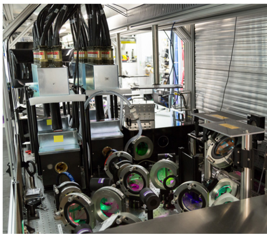
Figure 8. (Left) Picture of MEC Nd:glass laser system showing the 25 mm rod amplifiers. A laser pulse shaping system delivers about 4.5 J in 3 ns per beam on target at 527 nm. (Right) Examples of laser pulse shapes are shown for shock (blue) and ramp wave (red) compression experiments.
