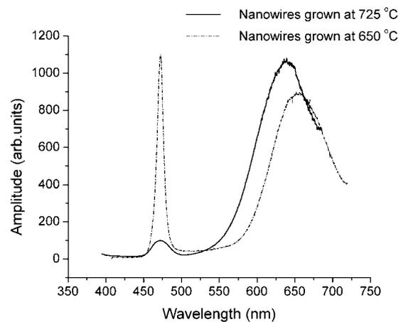
**Figure 4.** Typical PL spectra from ZnSe nanowires grown at 650 °C and 725 °C. The band edge emission intensity ( $\sim 463$  nm) decreases with increasing growth temperature while the broad deep defect-related emission (extending from 500 to 680 nm) increases.
