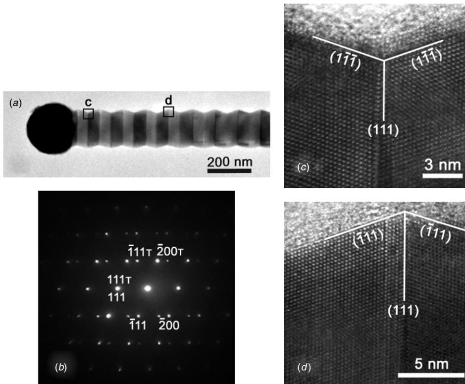
**Figure 3.** BF images (a) and (b) of a ZnSe nanowire with a large twinning periodicity and the corresponding electron diffraction pattern; HRTEM images (c) and (d) from the square-enclosed regions in (a).
