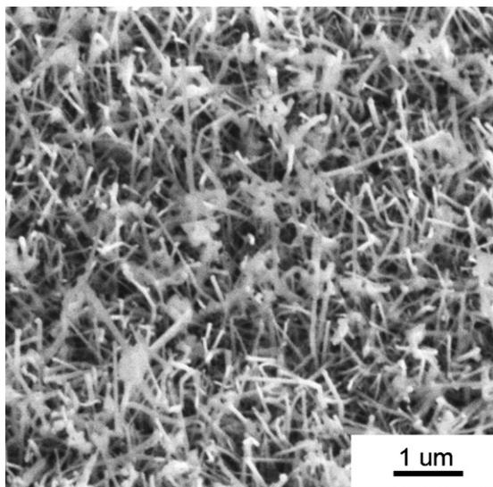
**Figure 1.** A typical SEM image of the ZnSe nanowires investigated.
