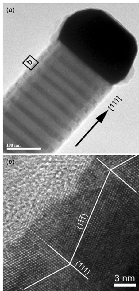
**Figure 2.** (a) A typical bright-field (BF) TEM image of a ZnSe nanowire with alternating black/light contrast; (b) HRTEM image from the square-enclosed region in (a).
