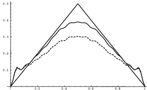
**Figure 6.** Solution of inverse eigenvalue problem with noisy data (3%), linear and quadratic approximations of the exact solution.
