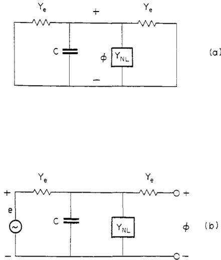
FIG. 4.—(a) Circuit model of the flute instability, including line-tying. (b) Circuit model for feedback stabilization of the flute mode at the ends.
