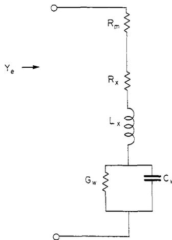
FIG. 3.—Equivalent circuit model for the mirror sheath, external plasma and endwall sheath.
