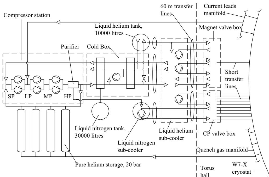
Figure 2. Layout of the W7-X refrigeration plant with warm sub-atmospheric compressor version.
