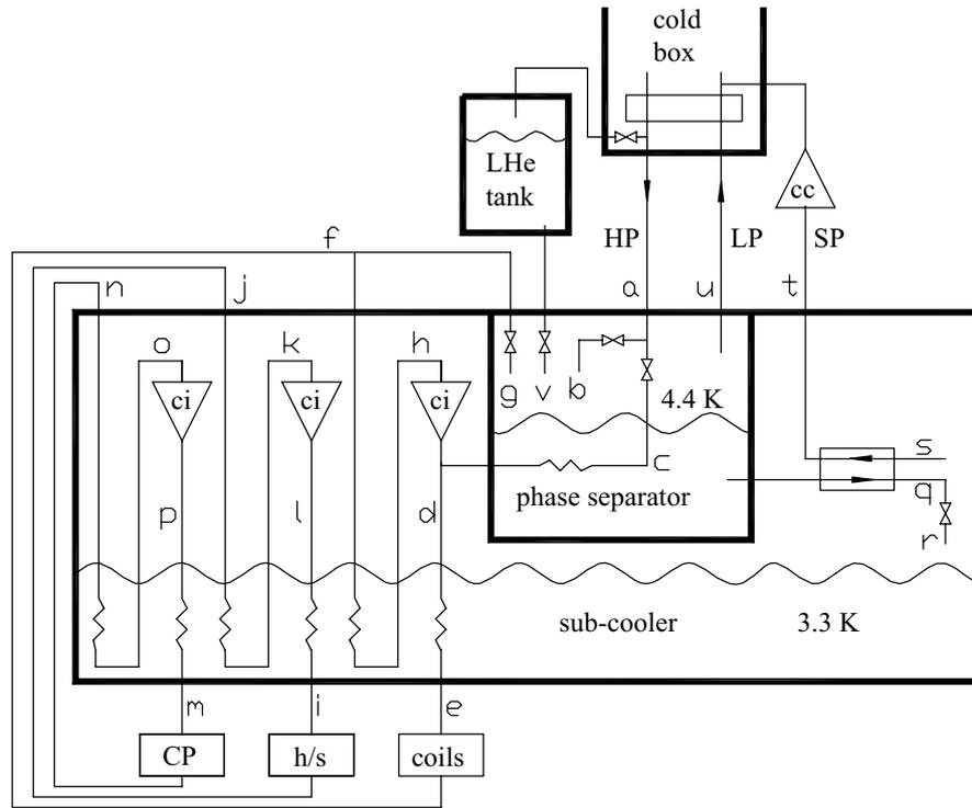
**Figure 3.** Basic sub-cooler and phase separator arrangement with cold SP compressor version. HP—high pressure stream; LP—low pressure stream; SP—sub-atmospheric pressure stream; cc—cold compressor; ci—cold circulator; CP—divertor cryo-pumps; h/s—housing and support circuit; coils—coils circuit.
