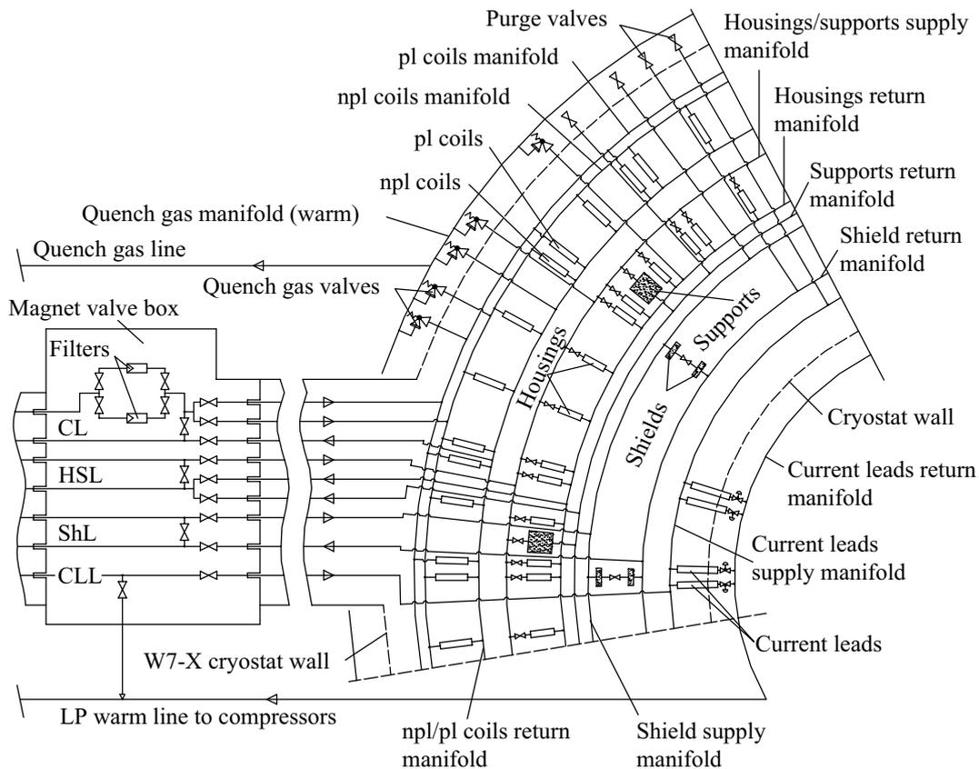
**Figure 1.** Components to be cooled and coolant supply of W7-X, module 3. CL—coils loop; HSL—hosings and support loop; ShL—shield loop; CLL—current leads loop.
