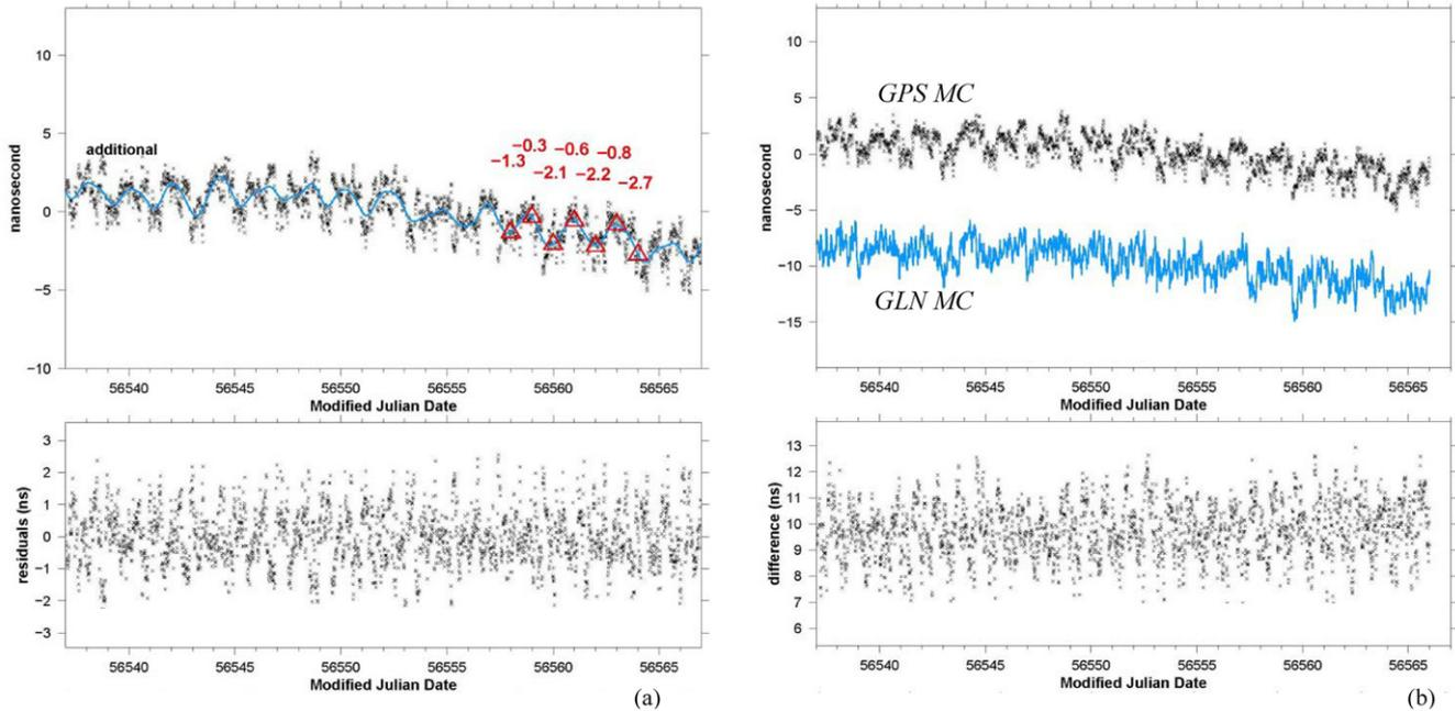
**Figure 3.** Example of a UTCr time link computation (a) and time link comparison (b). The top plots display the link results (a) and the two compared links (b) while the bottom plots display the residuals to a smoothing (a) and the difference of the two compared links (b), with all units in nanoseconds.
