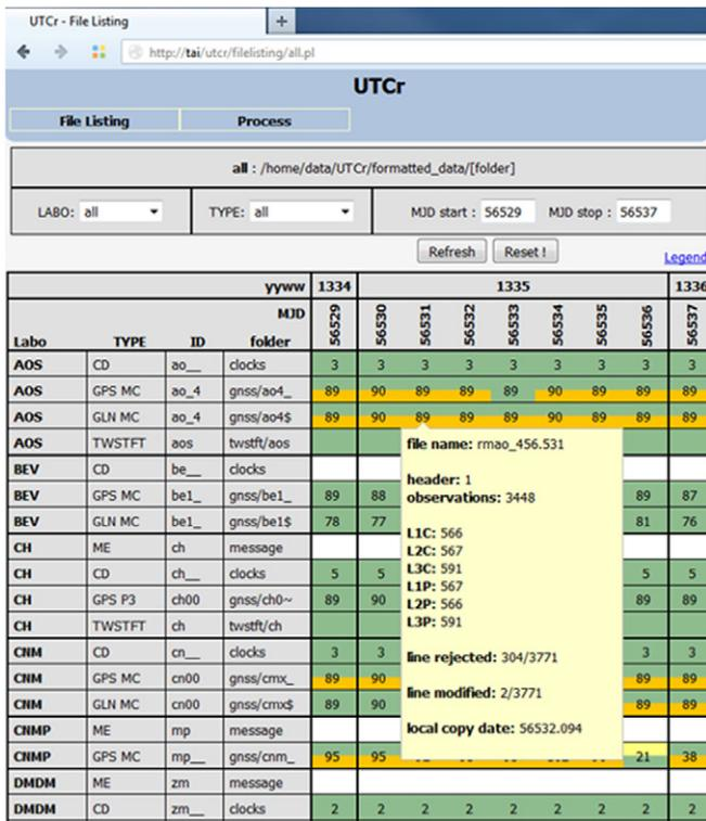
Figure 2. Example of automatic report showing the status of the recognized data files of UTCr week 1335. A pop-up window shows details on the content of one of the files.
