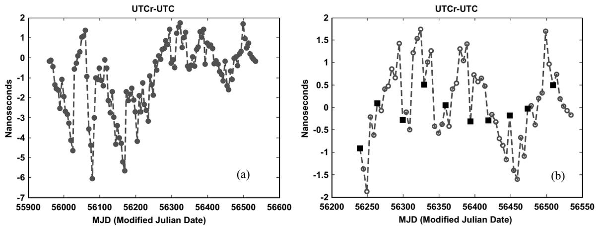
**Figure 4.** Comparison of UTCr to UTC: (a) from the beginning of the pilot experiment in February 2012 until August 2013 (19 months); (b) from the finalization of the procedure in November 2012 until August 2013 (10 months); in (b) filled squares indicate the first UTCr values immediately following a monthly UTC computation, i.e. following a steering of UTCr to UTC. See sections 3.4 and 4.1 for details.
