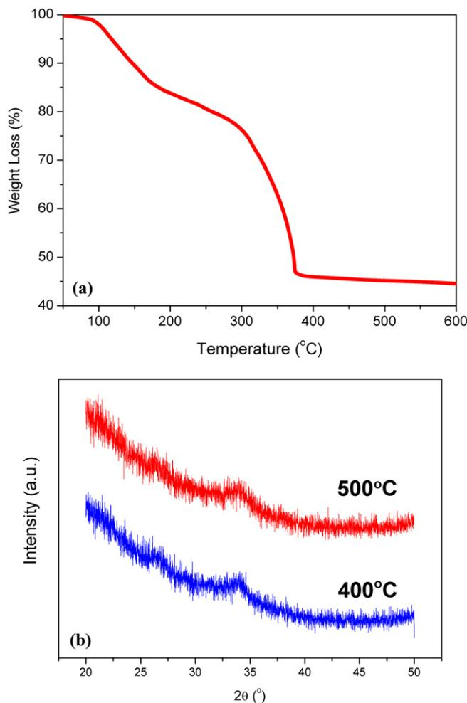
**Figure 1.** (a) TGA of the ZTO precursor solution at  $5\ ^\circ\text{C}\ \text{min}^{-1}$  heating rate in air and (b) the XRD pattern obtained from the ZTO thin film annealed at 400 and 500 °C for 1 h in air.
