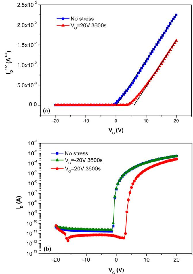
**Figure 5.** (a) Square root of the drain current versus gate voltage ( $I_D^{1/2} - V_G$ ) before and after gate bias stress at  $V_G = 20$  V for 3600 s and (b) the drain current versus gate voltage ( $I_D - V_G$ ) transfer characteristics under positive and negative gate bias stress for 3600 s with  $V_{DS} = 20$  V.
