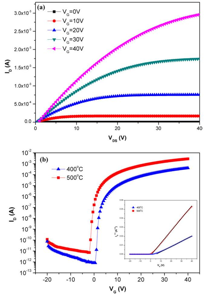
**Figure 4.** (a) Drain current versus drain-to-source voltage ( $I_D - V_{DS}$ ) output characteristics of the ZTO TFT annealed at 500 °C and (b) drain current versus gate voltage ( $I_D - V_G$ ) and the square root of the drain current versus gate voltage ( $I_D^{1/2} - V_G$ , inset) transfer characteristics of the ZTO TFT annealed at 400 °C and 500 °C with  $V_{DS} = 40$  V.
