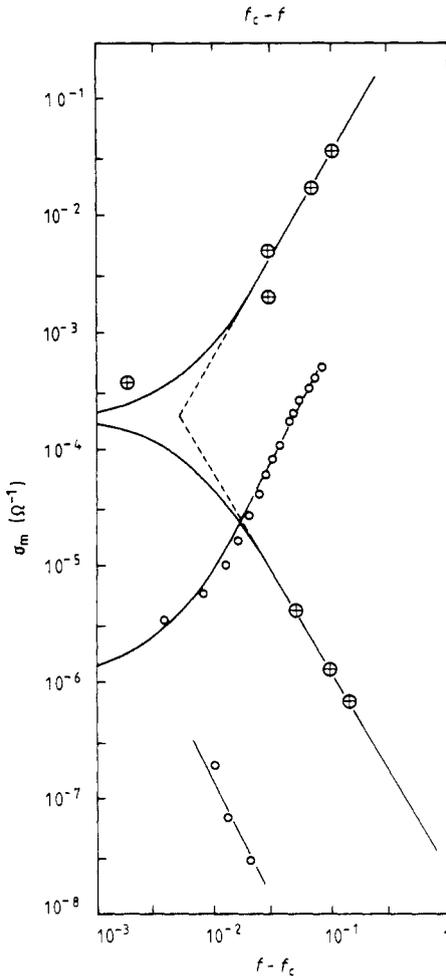
**Figure 2.** The conductivity of a gold ( $\oplus$ ) and a bismuth ( $\circ$ ) film as a function of  $f_c - f$  on the upper 'conducting' side and  $f - f_c$  on the lower 'insulating' side.  $f$  is the non-coated area fraction and  $f_c$  the critical value ( $f_c = 0.245$  (gold) and  $0.202$  (bismuth)). The full curves are equation (8) using the parameters given in the text. The broken lines are extrapolations from the dilute linear (or power law) linear regions.
