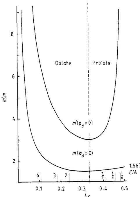
**Figure 1.** The exponents  $m$  and  $m'$  for random ellipsoids of revolution plotted against the demagnetisation coefficient  $L_c = L_b \neq L_a$ . These values are obtained by evaluating equation (23) in Meredith and Tobias (1962) in the limits  $\sigma_d = 0$  and  $\sigma_d = \infty$ .
