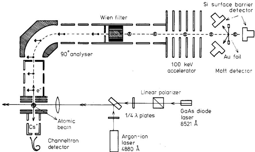
Figure 1. Experimental arrangement for measurements of ion count rate and electron spin polarization in the two-step photoionization of alkali atoms.
