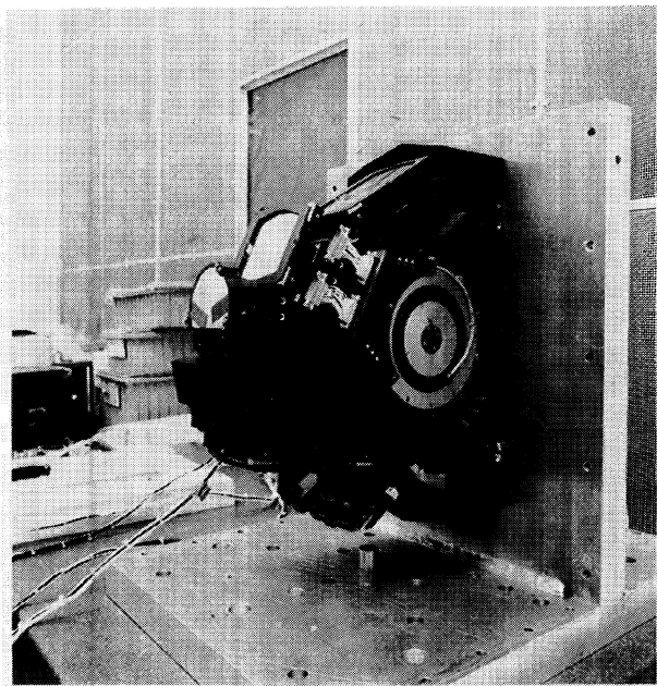
FIG. 4—The GHRS carousel with dummy optics, mounted on a test fixture. The GHRS echelle, first-order gratings, and target acquisition mirrors are mounted on the carousel and rotated into the correct position for observation. Courtesy of Ball Aerospace Systems Group.
