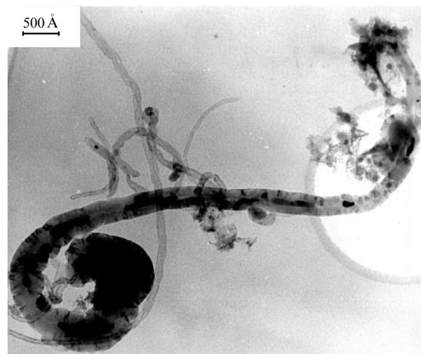
**Figure 9.** A micrograph of the filamentous carbon formed from methane on an Ni/Al<sub>2</sub>O<sub>3</sub> catalyst at 1023 K.
