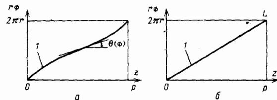
FIG. 7. 1—Development of the cylinder in a plane, which allows one to calculate the solid angle described by the vector  $\hat{\mathbf{k}}$ , with nonuniform winding (a) and with uniform winding for a light guide of length  $L$  (b).
