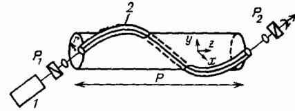
FIG. 6. Diagram of the apparatus of Tomita and Chiao.<sup>45</sup> 1—He-Ne laser,  $P_{1,2}$ —polarizers; 2—single-mode fiber light guide wound on a cylinder of length  $p$ .
