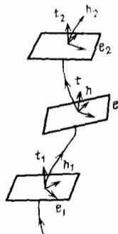
FIG. 4. The trihedron  $\{\mathbf{t}, \mathbf{e}, \mathbf{h}\}$  moving along a bent light ray;  $\mathbf{t}$ —tangent vector;  $\mathbf{e}$  and  $\mathbf{h}$ —unit vectors of the electric and magnetic fields.
