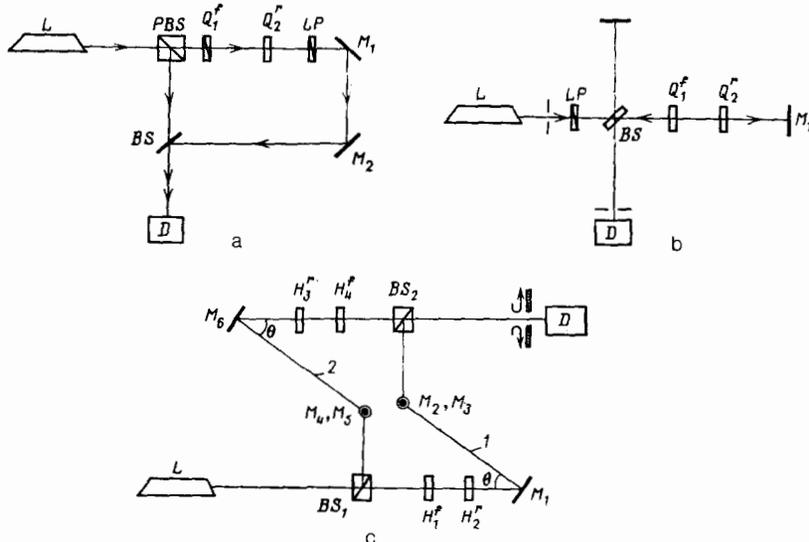
FIG. 15. Simplified diagram of laser interferometers used to measure the Pancharatnam phase in Ref. 54 (a), Ref. 61 (b), and Ref. 57 (c).  $L$ —laser,  $M_i$ —mirrors,  $BS_i$ —beam splitters,  $PBS$ —linearly polarizing splitter,  $LP$ —linear polarizers,  $Q_i^{\text{rot}}$  and  $H_i^{\text{rot}}$ —movable and immovable  $\lambda/4$  and  $\lambda/2$  phase plates, respectively,  $D$ —radiation receiver.
