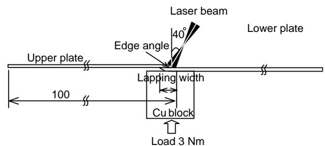
Fig. 7. Configuration of edge-line welding lap joint.
