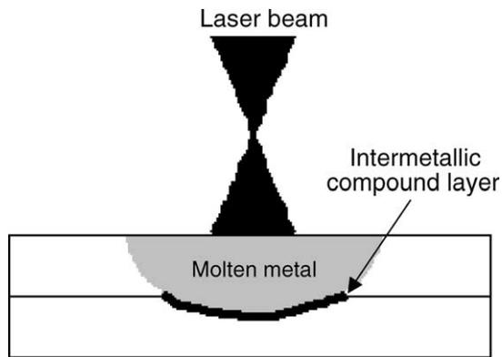
Fig. 1. Laser welding of lap joint.
