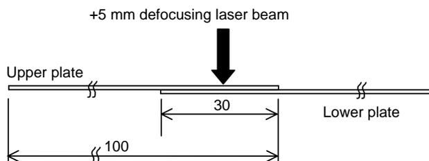
Fig. 3. Center-line welding lap joint.
