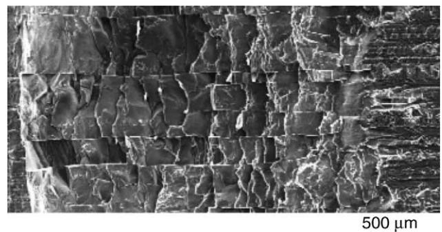
Fig. 10. Fracture surface of the joint at AZ31B (laser power, 3 kW; welding speed, 5 m/min; upper plate, A5052-O).
