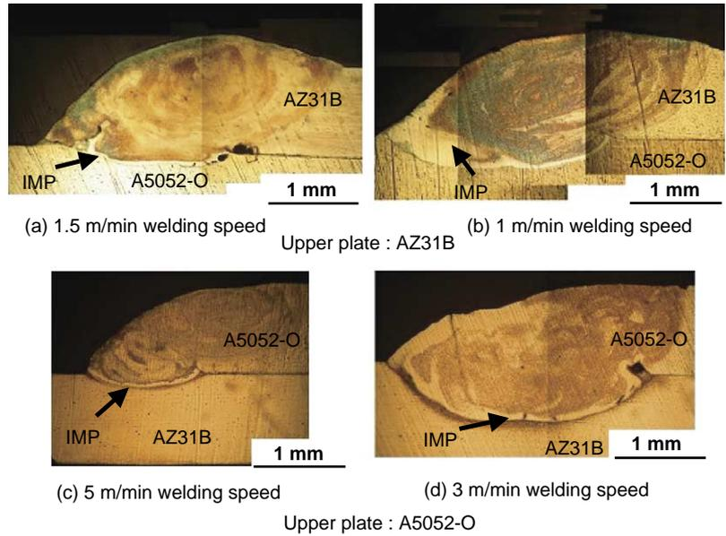
Fig. 8. Cross-sectional observations of edge-line welding lap joint.
