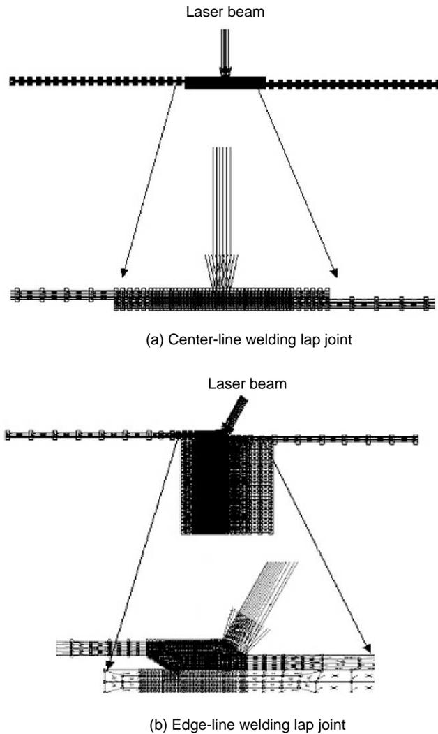
Fig. 5. FEM models. (a) Center-line welding lap joint; (b) edge-line welding lap joint.
