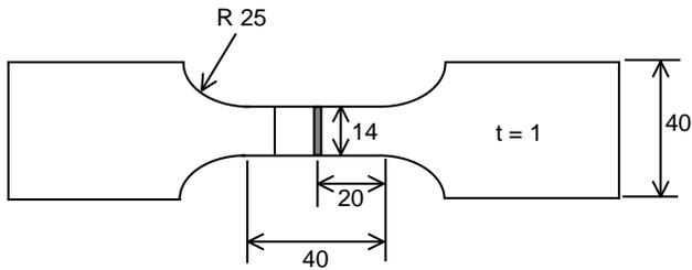
Fig. 2. Tensile–shear specimen.
