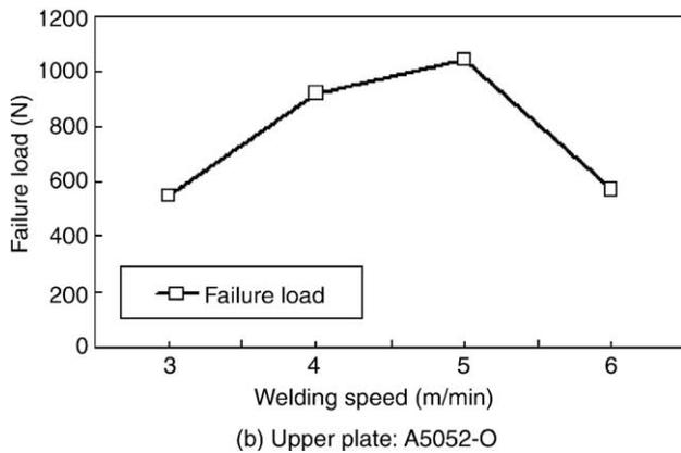
Fig. 9. Relationship between failure load and welding speed for edge-line welding lap joints.
