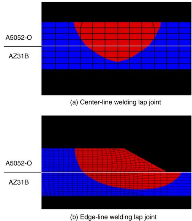
Fig. 6. The shapes of weld pool for center-line and edge-line welding at the same penetration depth. (a) Center-line welding lap joint; (b) edge-line welding lap joint.
