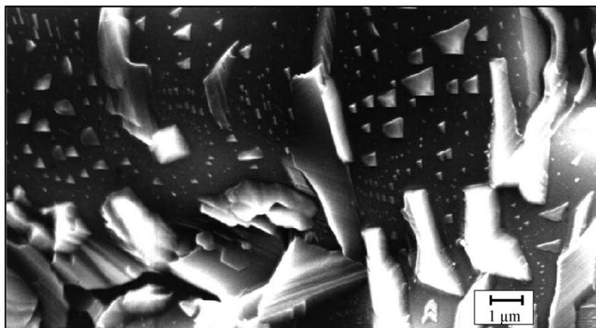
Fig. 8. SEM analysis of 3.5 wt% NiO/olivine calcined at 1400 °C.
