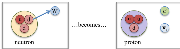
Figure 2.4. Beta decay is a weak interaction where a neutron turns into a proton. This happens when one of the down quarks in the neutron turns into an up quark by emitting a W boson. The W boson decays into an electron and an antineutrino.
