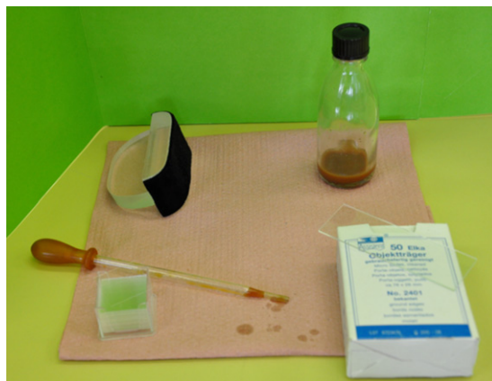
Figure 2.6. Object and cover glasses, a liquid crystal, a holder with velvet, and a dripping tube (Photo: Maja Pečar).
