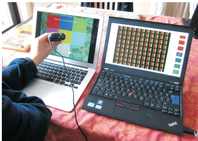
Figure 3.3. Observation of colours using a USB microscope. Use two portable computers, if possible; one screen to be studied and one screen on which to observe the magnification.
