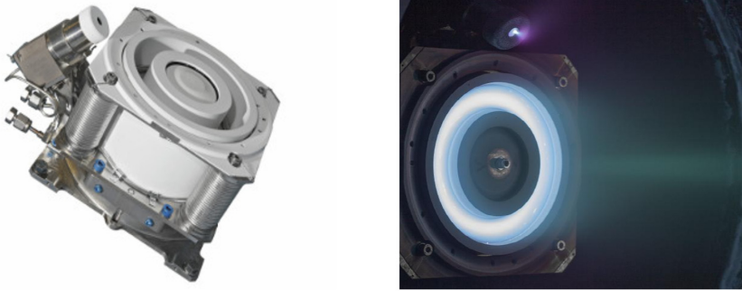
Figure 6.9. The Hall effect thruster PPS 1340-E on the left and operating in a vacuum tank in the right photograph. (Courtesy Safran-Snecma.) The hollow cathode is the cylinder attached to the equipment at its upper left and in operation is the bright dot of the right photograph.
