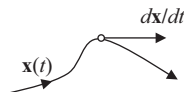
Figure II. A trajectory or phase curve \mathbf{x}(t) winding through the phase plane; the ‘velocity’ d\mathbf{x}/dt is tangent to this curve.
