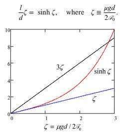
This is a transcendental equation for  $\zeta$  (and hence for  $\mathcal{T}_0$ ); from the plot of its both sides as functions of this variable (see the figure above) it is evident that the equation has a single positive root for any l/d > 1. Using the well-known asymptotic
