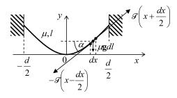
Solution: Let us introduce the Cartesian coordinates as shown in the figure above, with the origin at the lowest point of the rope. In equilibrium, the vector sum of the forces acting on each small rope fragment, of length dl, should vanish, so that for the vector  $\mathcal{F}$  of the rope tension force as a function of coordinate x we may write
