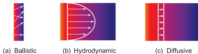
Figure 1.2. Schematic of phonon flux profile: (a) ballistic, (b) hydrodynamic and (c) diffusive. Reproduced with permission from [3]. Copyright 2015 Macmillan Publishers Ltd.
