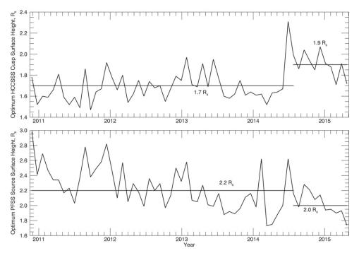
Figure 3. Interpolated optimum HCCSSS cusp surface heights (top plot) and PFSS source surface heights (bottom plot) in units of solar radii. These values give the best match to the IMF open flux for each CR. Also shown are reference lines corresponding to the overall values chosen for each epoch on the basis of minimum rms difference between IMF and coronal model (see Table 2).
