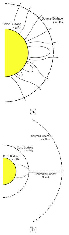
Figure 1. Diagram representations of coronal field extrapolation models. (a) The PFSS model assumes a "source surface" at which all magnetic field lines are open and radial. Moving the PFSS source surface to a lower height increases the open flux because it forces more higher-order structures to become open. (b) The HCCSSS model includes a "cusp surface," which we explain in the text. Moving this cusp surface in or out also affects the open flux calculated by this model.
