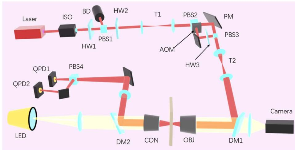
**Fig. 1.** (Color online) Schematic layout for DTOT (Laser, continuous-wave laser; HW, half-wave plate; PBS, polarizing beam splitter; BD, beam dump; AOM, acousto-optic modulator; PM, piezoelectric mirror; T, telescope; DM, dichroic mirror; OBJ, objective; SC, sample chamber; CON, condenser; QPD, quadrant photodiode; LED, light-emitting diode).
