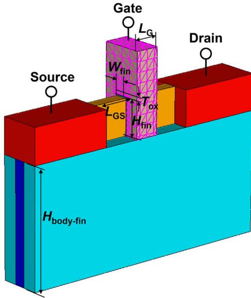
**Fig. 1.** (Color online) 3D schematic view of the proposed JL bulk-FinFET-based 1T-DRAM.
