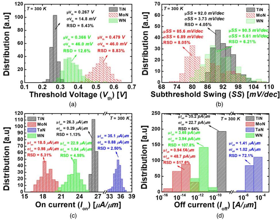
**Fig. 4.** (Color online) Histograms of the 200 samples of bulk-FinFET with (a) TiN, (b) MoN, (c) TaN and (d) WN gate materials based on the HK/MG technology.
