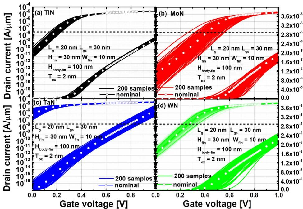
Fig. 3. (Color online)  $I_{ds}$ - $V_{gs}$  curves of the 200 samples of bulk-FinFET with (a) TiN, (b) MoN, (c) TaN and (d) WN gate materials based on the HK/MG technology. The current is normalized by the total fin width ( $W_{fin} + 2H_{fin}$ ).
