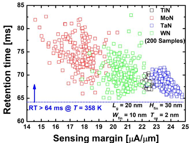
**Fig. 6.** (Color online) Comparison of retention time versus sensing margin for JL bulk-FinFET-based 1T-DRAMs with TiN, MoN, TaN and WN.
