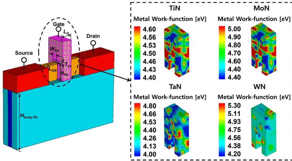
Fig. 2. (Color online) Examples depicting different orientations of grains in JL bulk-FinFET-based 1T-DRAM with TiN, MoN, TaN and WN gate materials.
