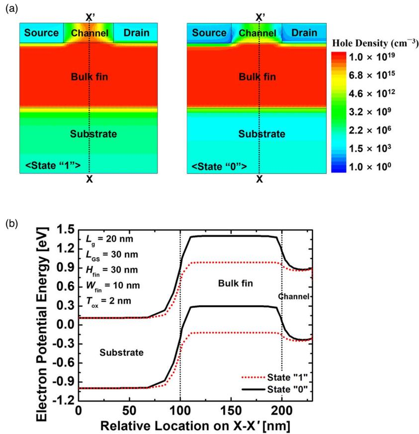
**Fig. 5.** (Color online) (a) Contour map of the hole density of the proposed 1T-DRAM cell in states "1" and "0." (b) Energy band diagram of the proposed 1T-DRAM cell in states "1" and "0." The energy band is extracted at the center of the channel.
