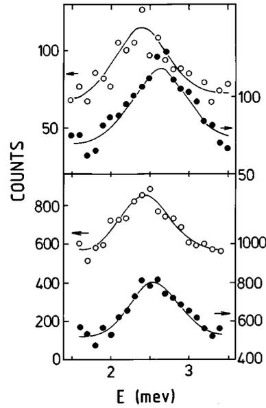
Fig. 2. – Constant- $Q$  scans for sample 1 (above) and sample 2 (below) at temperatures slightly above  $T_c$  (sample 1: 10 K, sample 2: 11 K; open circles) and below  $T_c$  (sample 1: 7 K, sample 2: 6.4 K; full circles).
