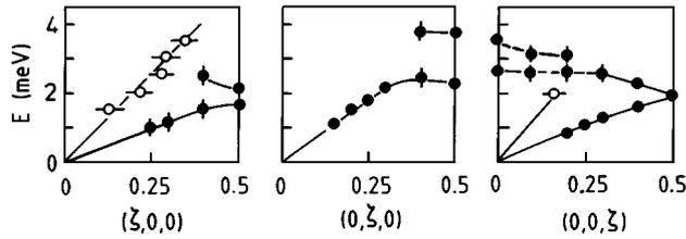
Fig. 1. – Phonon frequencies observed in longitudinal (L, open dots) and transverse (T, full dots) configuration at room temperature. Lines are a guide to the eye.
