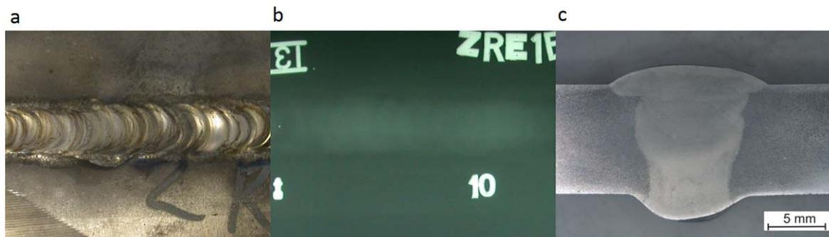
**Figure 3.** The results of the evaluation of the magnesium alloy welding joints for ZRE1 alloy as an example: (a) face of the weld, (b) X-ray pattern, (c) macrostructure.
