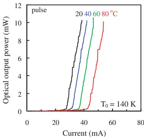
Fig. 3. Pulsed  $L-I$  characteristics of a  $c$ -axis stripe LD as a function of temperature.
