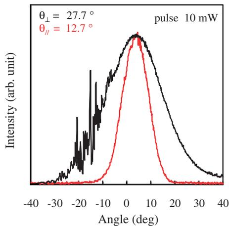
Fig. 4. Far-field patterns under pulsed operation at  $10\text{ mW}$ .
