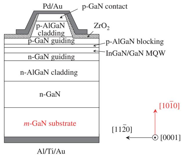
Fig. 1. Schematic drawing of the LDs with the stripe parallel to the *c*-axis.
