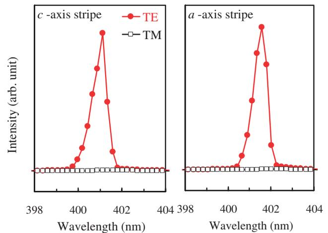
Fig. 6. Laser emission spectra of  $c$ - and  $a$ -axes stripe LDs under pulsed operation. The resolution of the monochromator was approximately  $0.2\text{ nm}$ .
