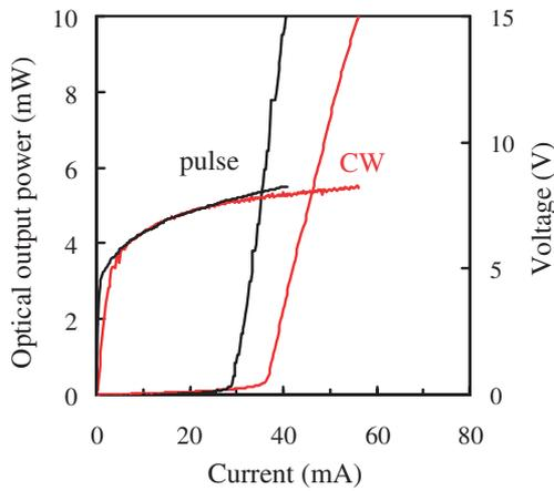
Fig. 2. Typical  $L-I$  and  $V-I$  characteristics of  $m$ -plane InGaN QW LDs with  $c$ -axis stripe under CW and pulsed operation at  $20^\circ\text{C}$ .
