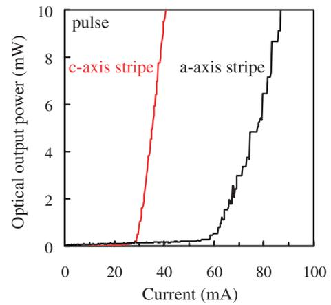
Fig. 5.  $L-I$  characteristics of  $c$ - and  $a$ -axes stripe LDs under pulsed operation.
