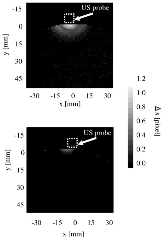
Fig. 6. Space-distortion images caused by (a) zirconia US probe (b) tungsten US probe.
