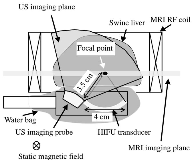
Fig. 3. Setup for MRI temperature measurement of tissue heated with MRI-compatible US applicator.
