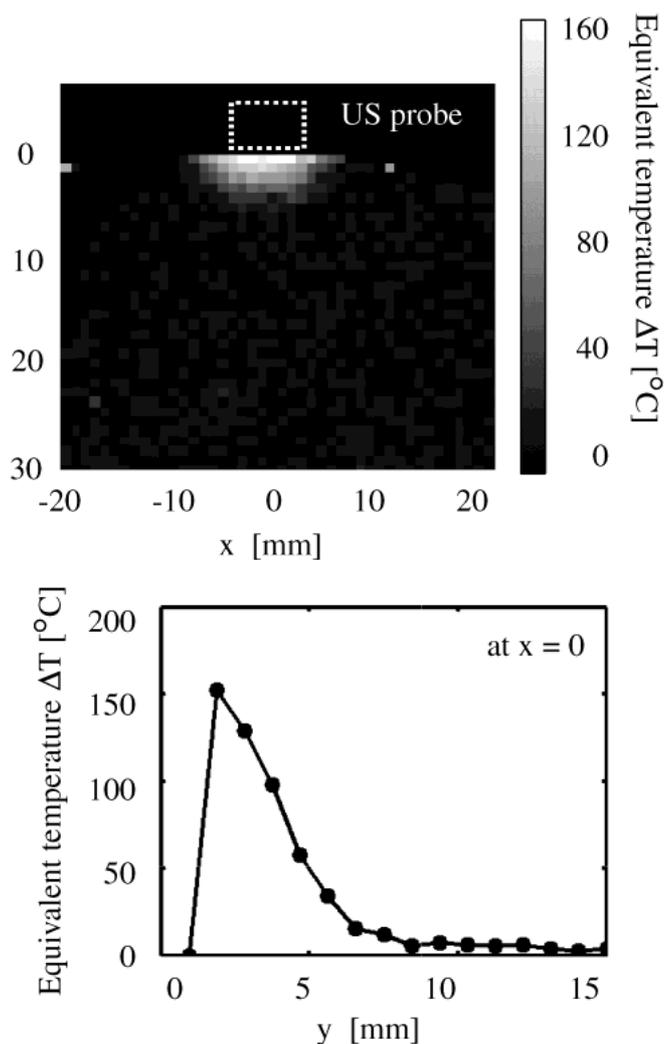
Fig. 7. Equivalent temperature change caused by the tungsten US probe.
