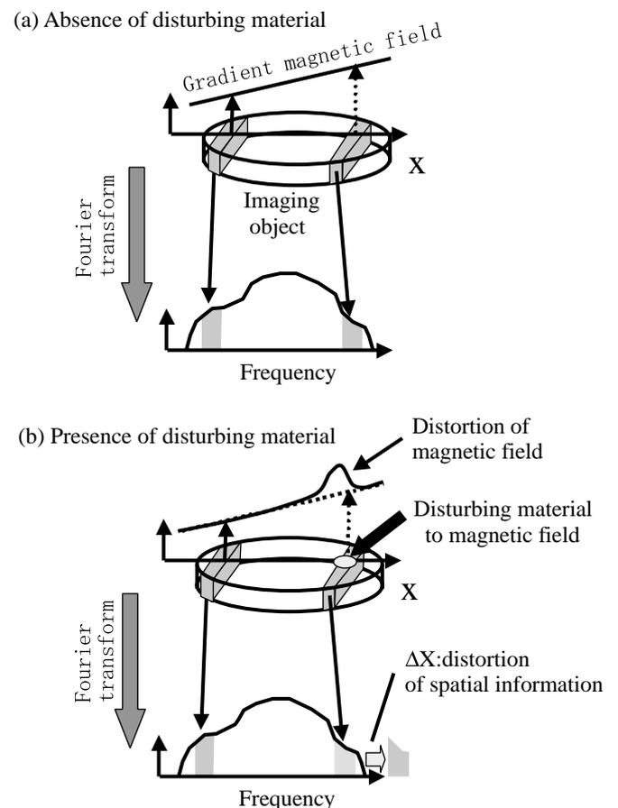
Fig. 5. Explanation for distortion of MR image caused by conventional US probe.
