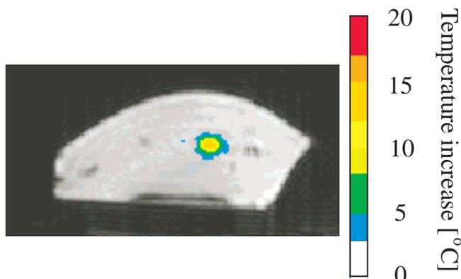
Fig. 10. Temperature map after radiation of HIFU.
