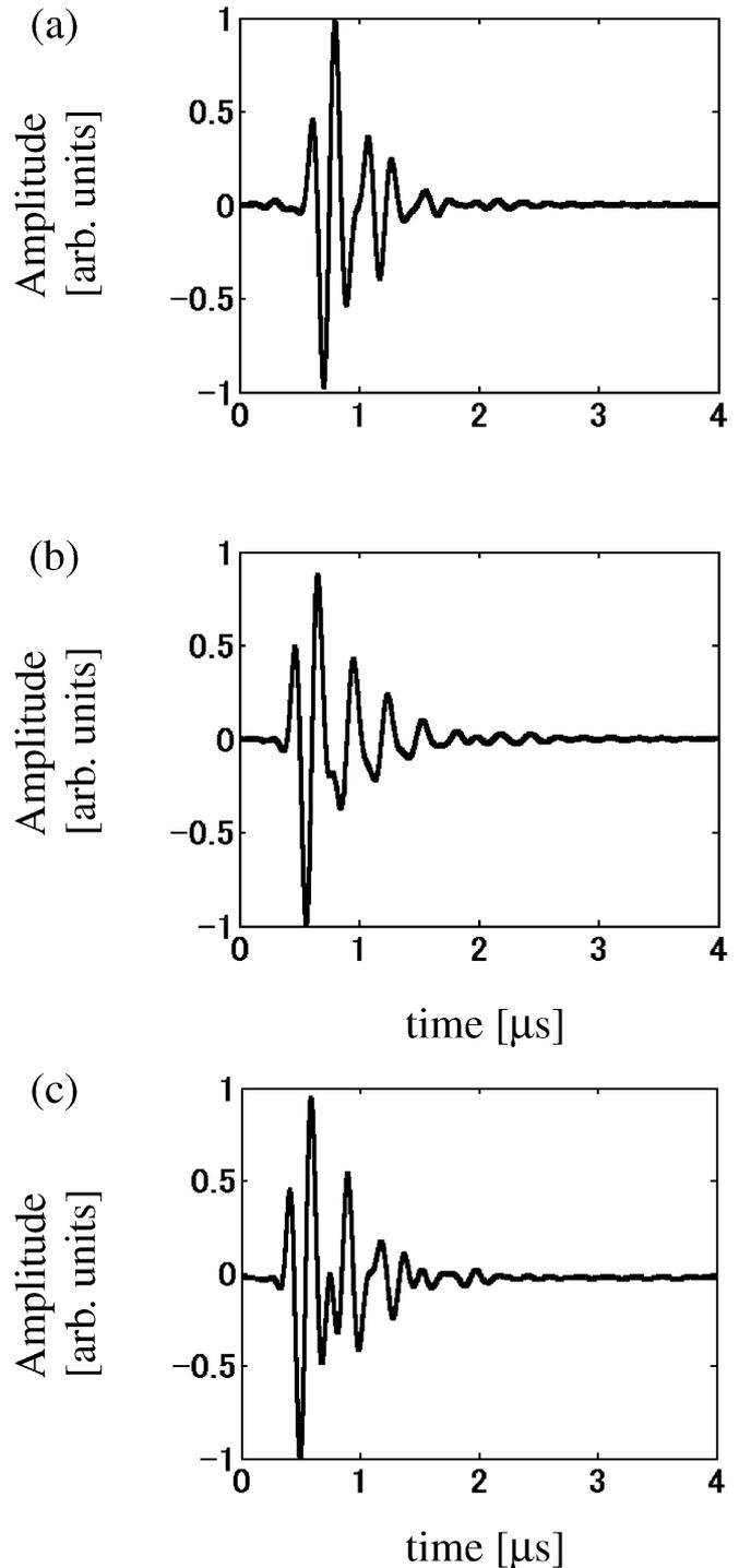
Fig. 9. Pulse responses of (a) conventional US probe, (b) zirconia US probe and (c) tungsten US probe.
