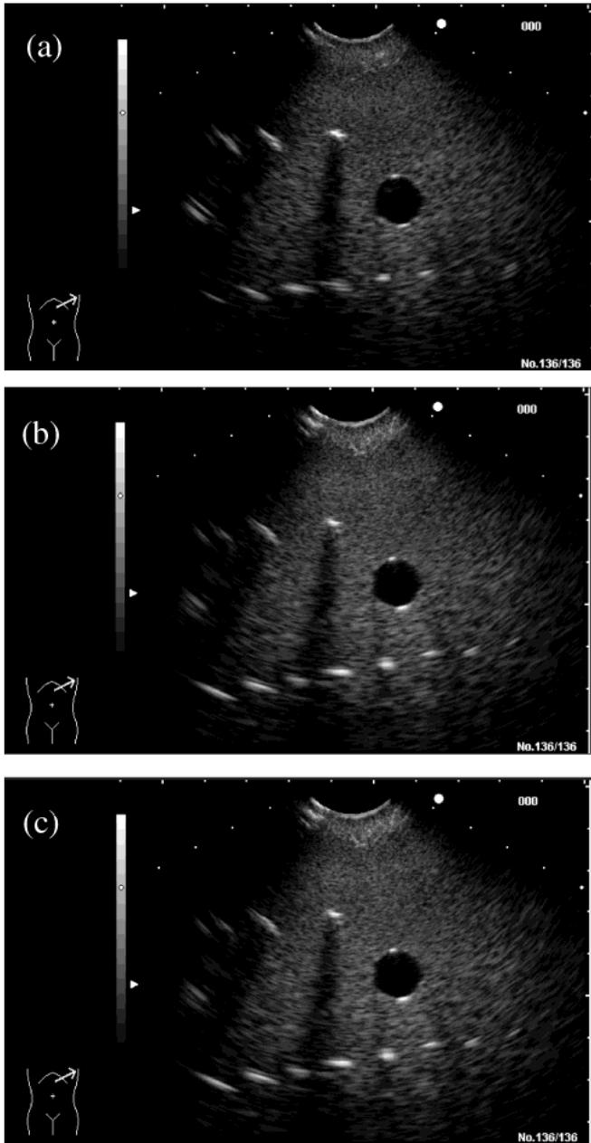
Fig. 8. B-mode images of US phantom taken by (a) conventional US probe, (b) zirconia US probe and (c) tungsten US probe.
