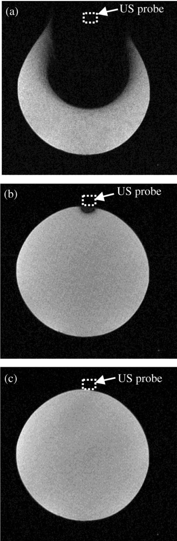
Fig. 4. Effects of MRI-compatible US probes on MR images. (a) Conventional US probe. (b) Zirconia US probe. (c) Tungsten US probe.
