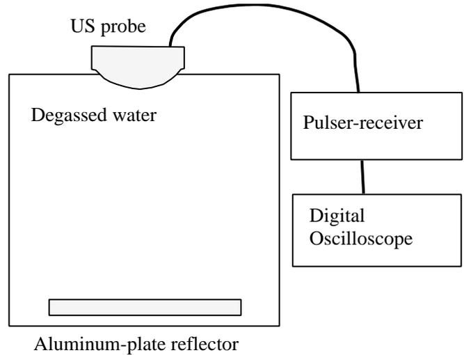
Fig. 1. Setup for measurement of the round-trip pulsewidth.
