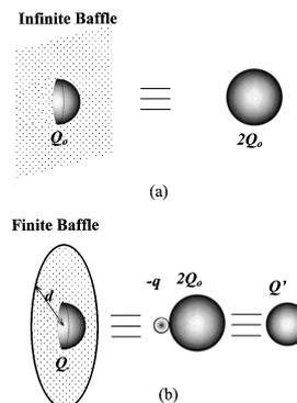
Fig. 1. Equivalent source strength of a point source with finite baffle.
