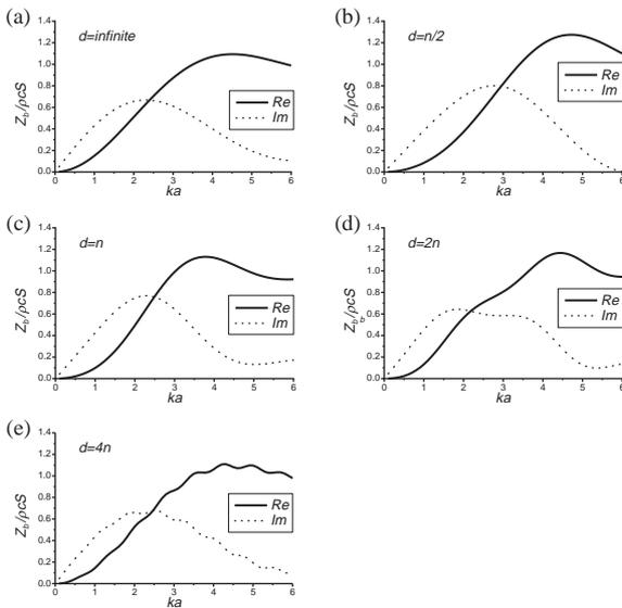
Fig. 3. Effect of baffle size on radiation impedance of rectangular vibrating surface.
