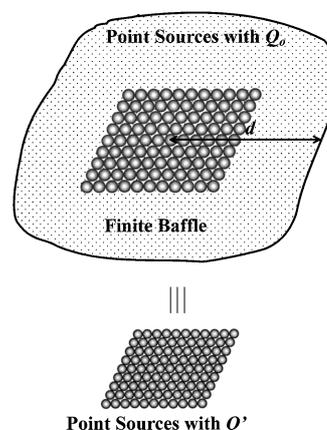
Fig. 2. Equivalent source strength of rectangular piston source with finite baffle.
