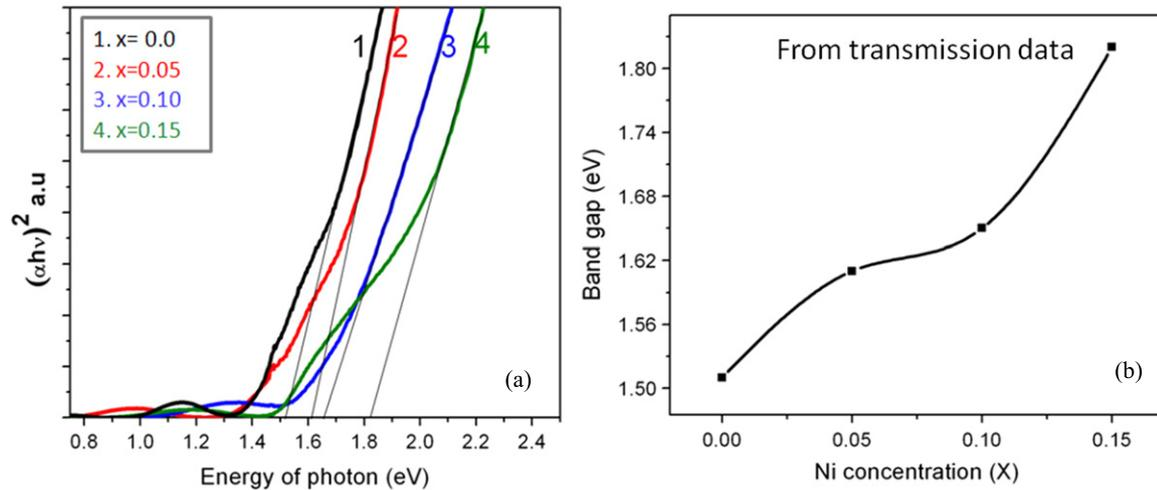
**Figure 8.** (a) Band gap calculation from transmission data. (b) Variation of  $E_g$  with Ni concentration.
