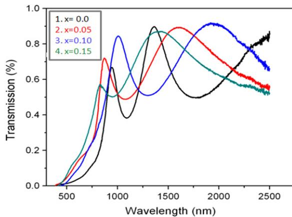
**Figure 7.** Transmission spectra of Cd<sub>1-x</sub>Ni<sub>x</sub>Te thin films.
