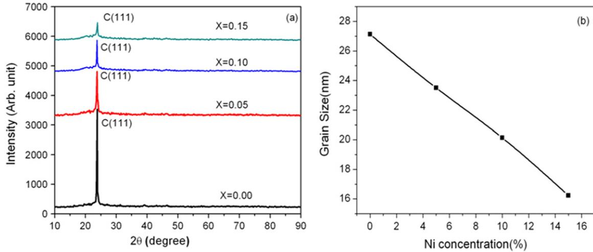
**Figure 1.** (a) XRD spectra of  $\text{Cd}_{1-x}\text{Ni}_x\text{Te}$  at various Ni compositions (b) grain size variation as a function Ni composition.
