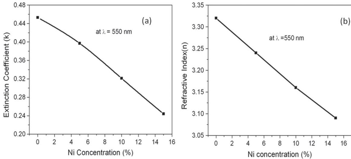
**Figure 5.** (a) and (b) shows the change in *n* and *k* values as a function of Ni concentration, respectively.
