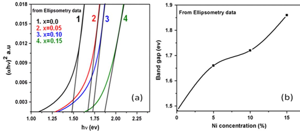
**Figure 6.** (a) Band gap ( $E_g$ ) as a function of photon energy (b)  $E_g$  variation with Ni concentration.
