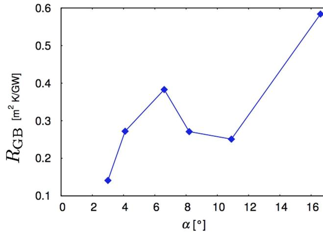
**Figure 6.** Predicted grain boundary thermal resistance  $R_{GB}$  as function of the tilt angle  $\alpha$  defining the structure of the grain boundary (see figure 1(b)).
