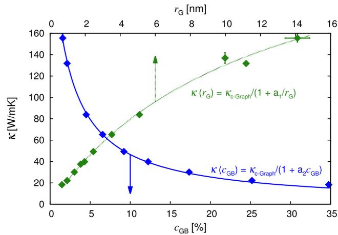
**Figure 7.** Predicted room-temperature thermal conductivity  $\kappa$  of nanocrystalline graphene as a function of the concentration of atoms in the grain boundaries  $c_{GB}$  (blue solid line), and of the average radius of gyration of the graphene grains  $r_G$  (green dotted line). Simulations correspond to samples as long as 200 nm.
