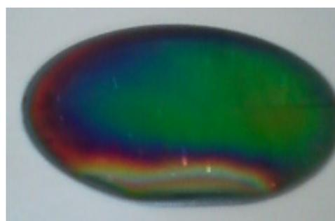
Figure 5. Fabricated 1D-NPSMC structure.
