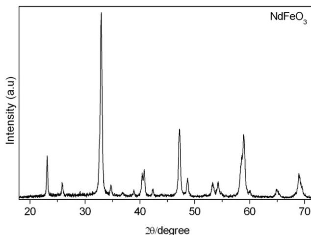
**Figure 2.** XRD pattern of the powder  $\text{NdFeO}_3$  synthesized by the sol-gel citrate technique.
