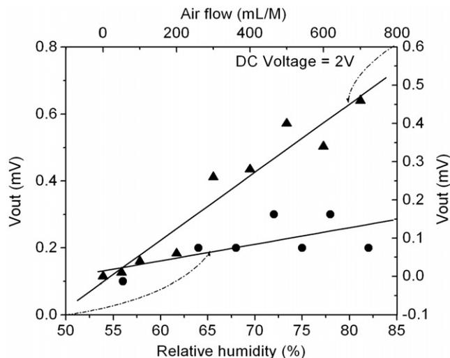
**Figure 6.** The influences of relative humidity (circular symbols) and air flow rate (triangular symbols) on the cross-sensitivity of the sensor at an applied voltage of 2 V.
