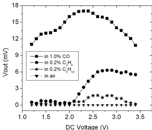
**Figure 4.** The gas response ( $V_{out}$ ) dependences on applied voltage (dc voltage) in the air with a trace of some reducing gases.
