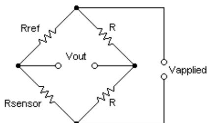
**Figure 1.** The electrical circuit for the operation of a catalytic gas sensor.
