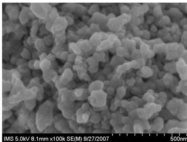
**Figure 3.** SEM image of the powder  $\text{NdFeO}_3$  calcined at  $700^\circ\text{C}$ .
