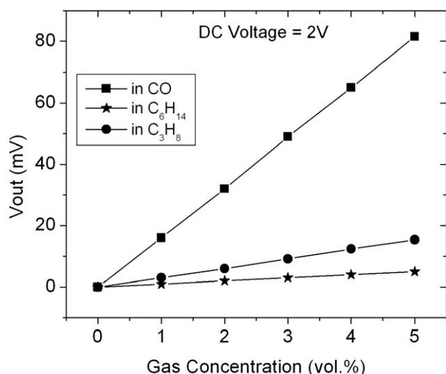
**Figure 5.** The characteristic of the response ( $V_{out}$ ) to gas concentrations of CO,  $C_3H_8$  and  $C_6H_{14}$ .
