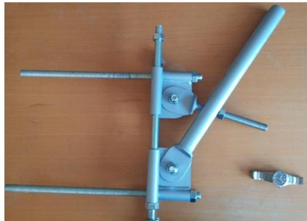
**Figure 15.** The created optimized Lever Anchor (with the wrist watch in the bottom right corner as a scale).
