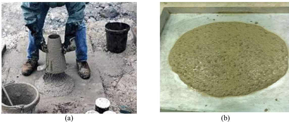
Figure 1. a) Abram's cone; b) Abram's cone outflow view (for its diameter measurement).
