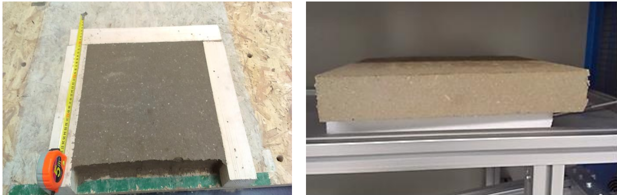
Figure 2. Left: A freshly removed sample, Right: A sample after curing until reaching a constant mass.
