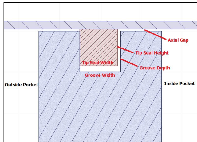
Figure 4: A typical cross section of tip seal leakage path.
