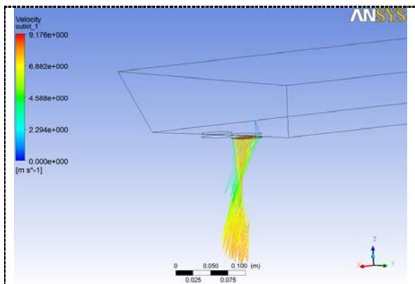
**Figure 8.** Airflow rate of outlet 1 for deflector 90°.
