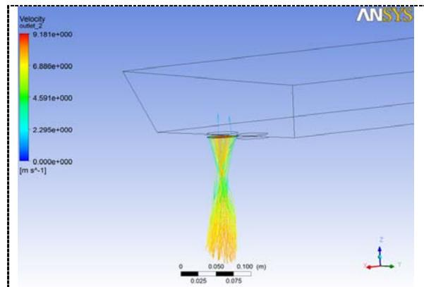
**Figure 9.** Airflow rate of outlet 2 for deflector at 90°.
