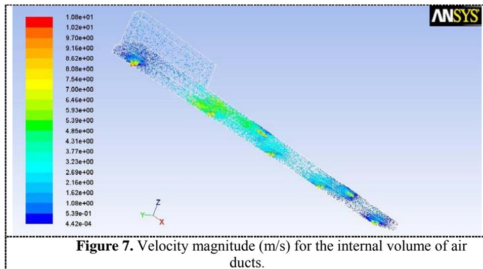
**Figure 7.** Velocity magnitude (m/s) for the internal volume of air ducts.
