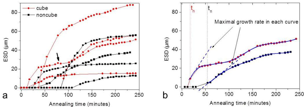
Fig. 3 Selection of measured growth curves. a) Growth curves of 4 cube grains and 4 noncube grains. The arrow marks a stagnation period. b) Examples explaining how the nucleation time  $t_n$  and maximal growth rates  $g$  were determined.  $t_n$  was the time when the grain was first observed. Each growth curve was fitted using a spline function (the blue curve), and the largest slope of the fitted curve was used as  $g$ .
