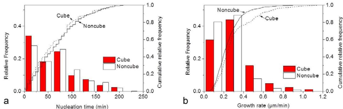
Fig. 4 Distributions of nucleation times  $t_n$  (a) and maximal growth rates  $g$  (b) for cube and noncube grains that are larger than  $10 \mu\text{m}$  at the end of the measurement. The histograms show the relative frequencies, and the curves show the cumulative relative frequencies. The bin widths are 30 min and  $0.2 \mu\text{m}/\text{min}$  for a) and b) respectively.
