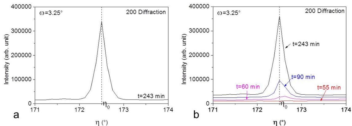
Fig. 1 Example showing the process of peak identification. a) The peak was first identified from the diffraction image collected during the last 30° rotation. The peak position ( $\omega, \eta_0$ ) were noted. b) The same peak at earlier times was found according to the peak position. This peak first appeared at  $t=60$  min, and its intensity increased with time. For clarity, the peak is only plotted for a few time steps.
