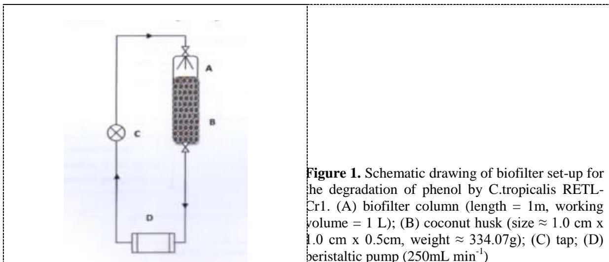
**Figure 1.** Schematic drawing of biofilter set-up for the degradation of phenol by *C.tropicalis* RETL-Cr1. (A) biofilter column (length = 1m, working volume = 1 L); (B) coconut husk (size ≈ 1.0 cm x 1.0 cm x 0.5cm, weight ≈ 334.07g); (C) tap; (D) peristaltic pump (250mL min<sup>-1</sup>)
